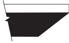
NSS Bevel "G" 2mm PVC Edge with Black Foil on Melamine Chassis
